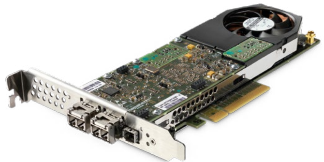
Example: NT20E2-PTP frame time stamps on two ports on one accelerator
